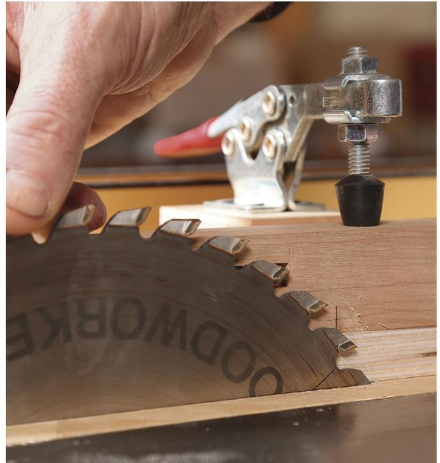
**Set the fence.** With the platform of the sled against the table-saw fence, slide the fence over so the sled just fits between it and the blade, as if you were ripping a board to the width of the jig (left). To check the setting, McLaughlin scrapes the leg with the blade to make sure the cut begins at his line or just past it.
