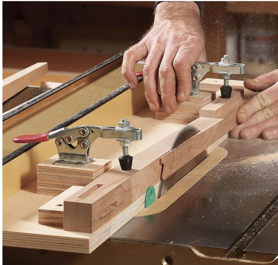
**Offcut simplifies second rip.** After one side has been tapered, the toggle over the bottom of the leg will no longer touch when snapped into position. A spacer shim made from the initial tapered cutoff and cut to length quickly solves this problem.
