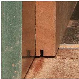
**Step 2: Cut the bevel.** Place the rail face down on the sawtable with its bottom edge against the fence, and set the blade to 40°. Cut a bevel to the previously cut kerf.
