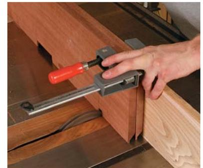
**Step 3: Dado the stile locations.** Mark the position of each stile's outside edges along the top of each rail. Turn the rails upside down, clamp them together, and hold them against a fence attached to a miter gauge. Cut 1/16-in.-deep dados.
