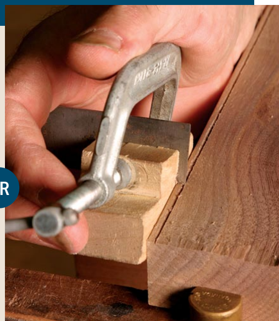
A low-tech method. A scratch stock made from a block of wood and a piece of scraper blade is an efficient way to create small amounts of beading.
