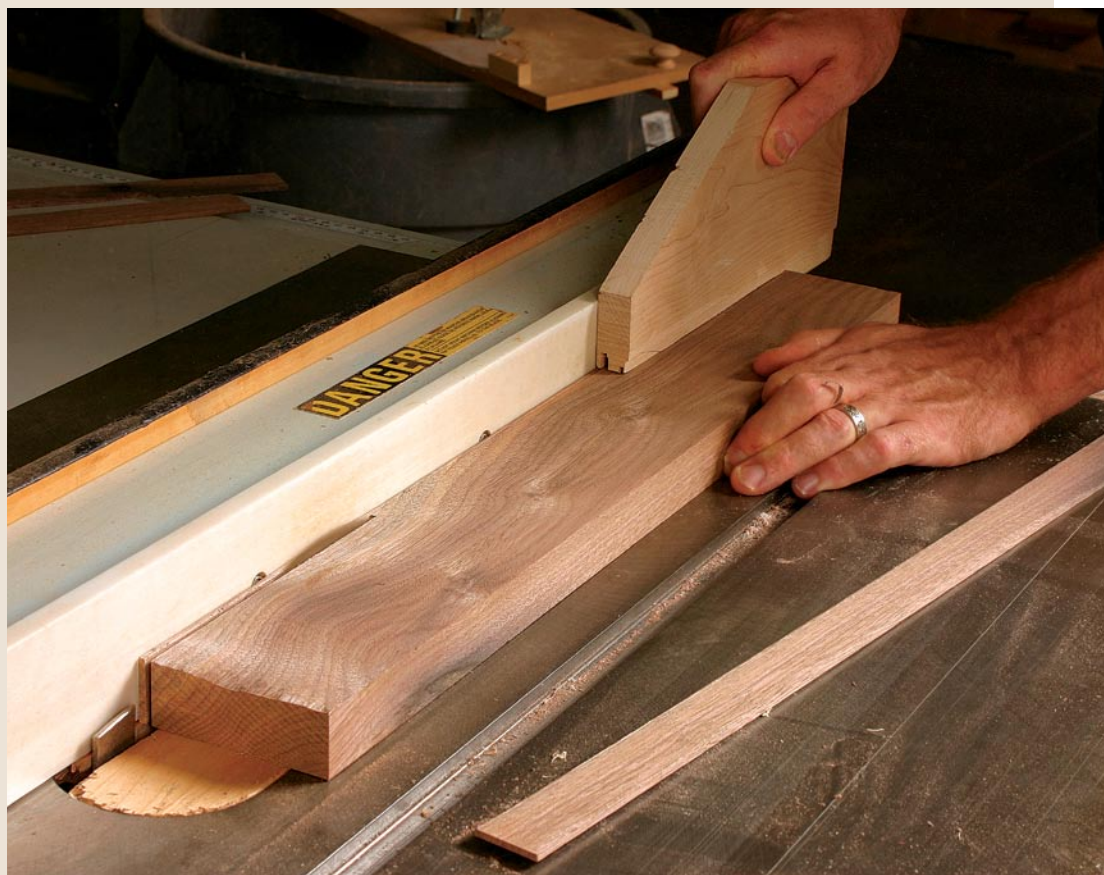
Rip the beading. After the bullnose profile has been routed or scratched, rip the beading to width on the tablesaw. A splitter prevents saw-burn marks on the sides of the beading.
