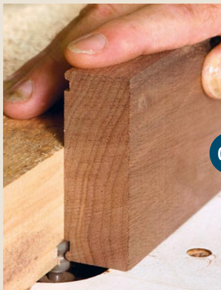
Router-cut beading. The fastest way to cut large amounts of beading is with a bullnose bit in a router table. Set the bit within a sacrificial fence.
